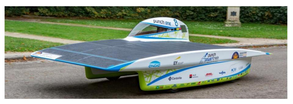
The Punch One Solar Car was produced using carbon fiber prepregs impregnated with bio-based epoxy resins to develop carbon fiber composite material for car body with 18% bio-content.
